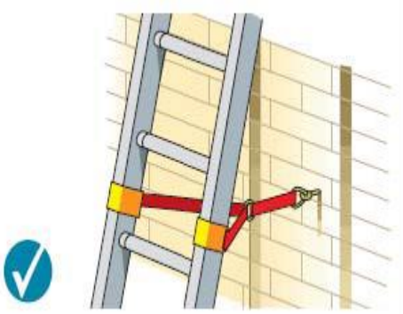
Tying near the base
