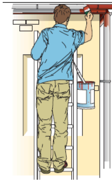
Maintaining 3 points of contact
